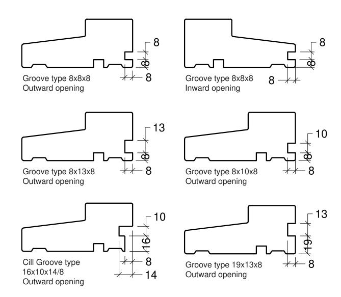
Grooves are standard for both alu and wood frame profiles.
